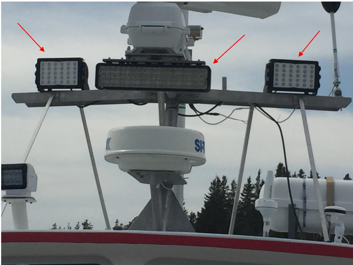
**Figure 1- Typical installation of forward-facing LED lights, noted with red arrows.**
