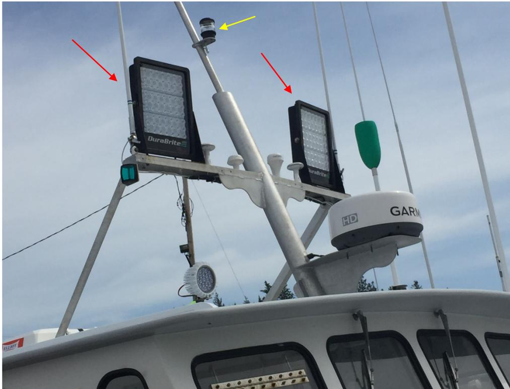
Figure 2- Forward-facing LED lights (red arrows) may obscure navigation lights (yellow).
